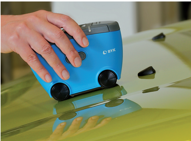
Measurement of surface quality (BYK, Wave Scan Dual)
