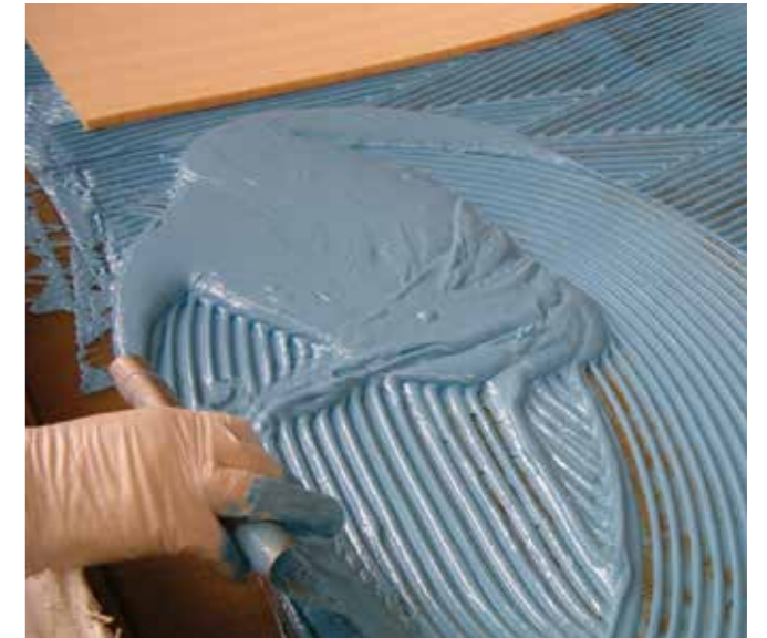
Processing of BÜFA®-Bonding Paste
