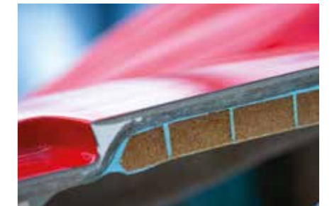
Different Bondings with BÜFA®-Bonding Pastes
