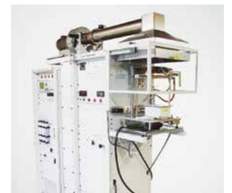
Cone calorimeter for investigating fire behaviour
