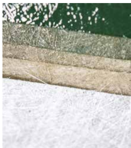
Laminate layer structure
