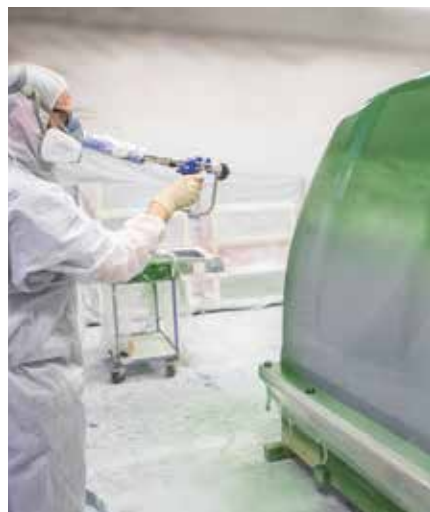
Applying gelcoat by spraying
