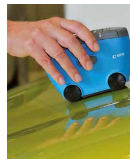
Measuring surface quality (Wave Scan Dual)
