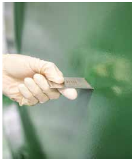
Measuring layer thickness
