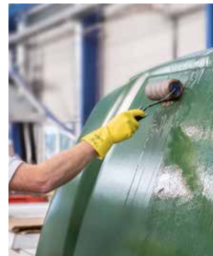
Pre-application of the 1. Layer resin
