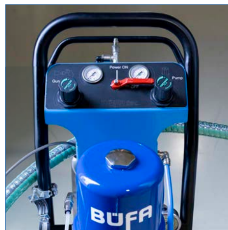
Panel de control
