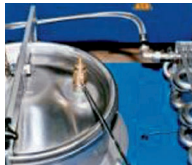
Safety valve in the container lid
