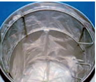
No steam pipe in the boiling tank
