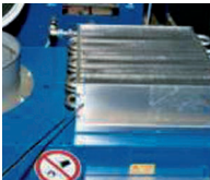
Air cooled, stainless steel condenser
