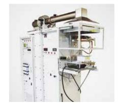
Cone calorimeter for investigating fire behaviour
